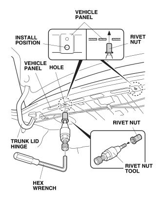
2. Open the trunk lid. Insert the rivet nut into the hole in the vehicle panel, and install the hex wrench on the rivet nut tool.
